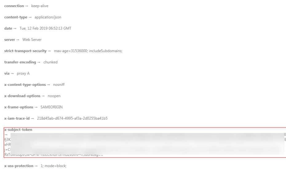
Figure 3-1 Header fields of the response to the request for obtaining a user token
